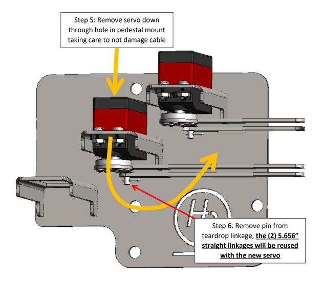
Step 7: Install new servo and secure using reverse of steps 5 & 4. Pin (2) 5.656" straight linkages to new servo using reverse of step 6.
